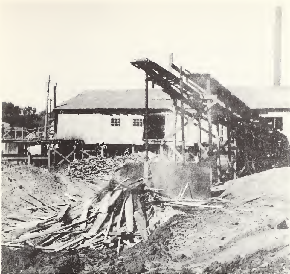
Figure 3.--Slabs and edgings are sometimes difficult to dispose of. Pulp mills will not accept them because they contain too high a proportion of bark. This mill is burning slabs and edgings to get rid of them.
